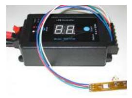
Most controllers have an input for 12 or 24 volts DC and an output for "R,G,B,+", known as "red" "green" "blue" and "12v positive".
