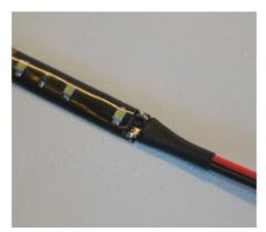
We recommend using a 1 inch section of  $\frac{1}{2}$ " heat shrink tube over the ends of your leads. A second section of  $\frac{1}{2}$ " heat shrink should then be applied over the remaining exposed leads/connection; finishing the waterproofing process. We have found that this reinforces and secures the soldered leads and LED Flexible Ribbon connection.
