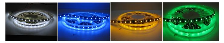
The Flexible Ribbon strip runs off **12 volts DC** (Direct Current) only. 24vDC is custom ordered. Observe polarity of Positive (+) and Negative (-) when connecting the power source. If the unit does not light, reverse the polarity and try again. You will not damage the LED Flexible Ribbon strip with connecting the 12vDC power source reversed; it simply will not light.
