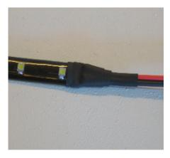
Multiple strips and/or colors can be connected together. Individually powered strips should always be connected in parallel (directly back to the 12vDC power source or main feed. Do not exceed six 5-Meter spools total length (30M – Single/Static color).
