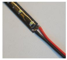
You will need to solder leads to the piece(s) to power them with your 12vDC supply. Using a low wattage soldering iron and electronic grade solder, attach you leads with solder to the Positive (+) and Negative (-) copper solder dots on your next piece.
